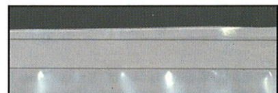
Barrier packaging materials with 3/4" wide flat seals are used for military and many other packaging applications.
