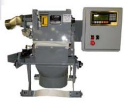
A typical application would utilize a GWD Wildcat digital scale or a GWM Wolverine mechanical scale for 20 to 110 lb bag weights; or a SMNW Falcon scale for 1 to 20 lb bag weights.
