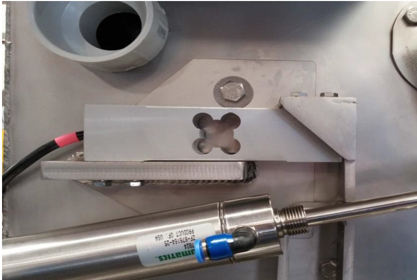
Photograph B - Permanent load cell and correct mounting position
