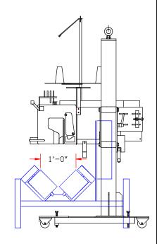
V CONVEYOR (BC12V) V CONVEYOR 12'0" LONG WITH SEWING PEDESTAL WITH SWING-AWAY FEATURE AND PHOTO EYE FOR START/STOP OF SEWING HEAD
