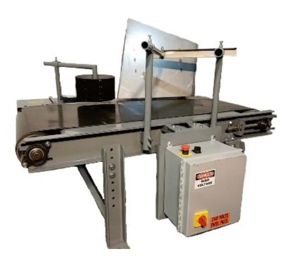
The KD5 Knockdown Bag Turning Conveyor will receive bags standing up, knock the bags down and turn the bags so that they are laying on either the front or back side and exit the conveyor bottom first. This conveyor is used for feeding flattening conveyors, miscellaneous printing systems or whenever the position of the bag is critical prior to palletizing.
